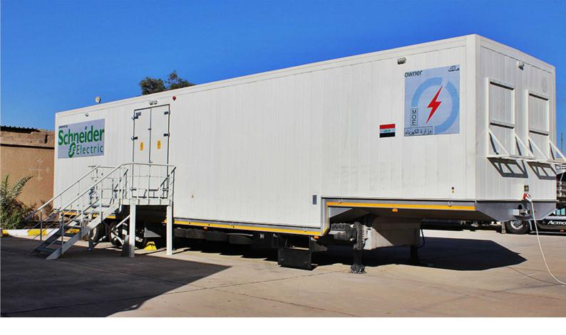
Mobile substations are a perfect solution for providing temporary connection to the main electrical grid, for temporary feeding.
